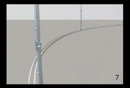
**5-7** Unfold the center support and bolt them to the lower horizontal frame section according to the labeling with the enclosed wing screws.
