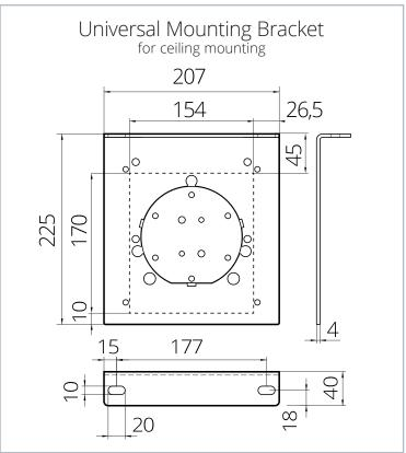
THE BRACKETS OF THE PROJECTION SCREEN MUST BE MOUNTED FORCE-FIT AND POSITIVE-FIT TO THE CEILING CONSTRUCTION! DO NOT PUT ADDITIONAL MECHANICAL LOAD ON THE CASING! THE MOUNTING MUST ENSURE THAT NO DISTORTION CAN ARISE!
