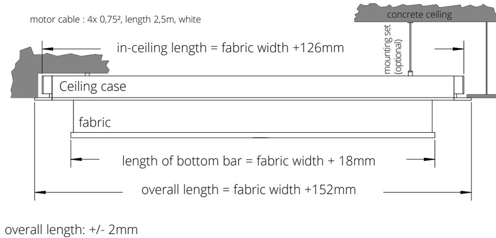
The recessed ceiling case can be pre-installed during building works.
