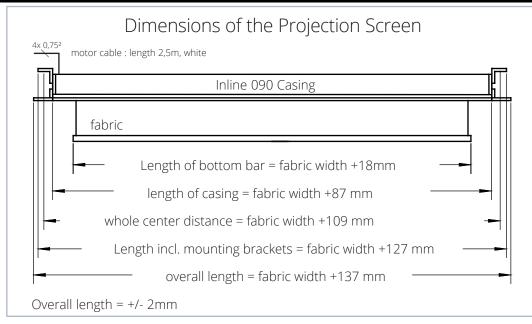
All projection screens in system Inline are available as projection screens for ceiling integration. The clips-brackets on either sides of the screen are stackable to allow convenient access to the screws for mounting and servicing.
