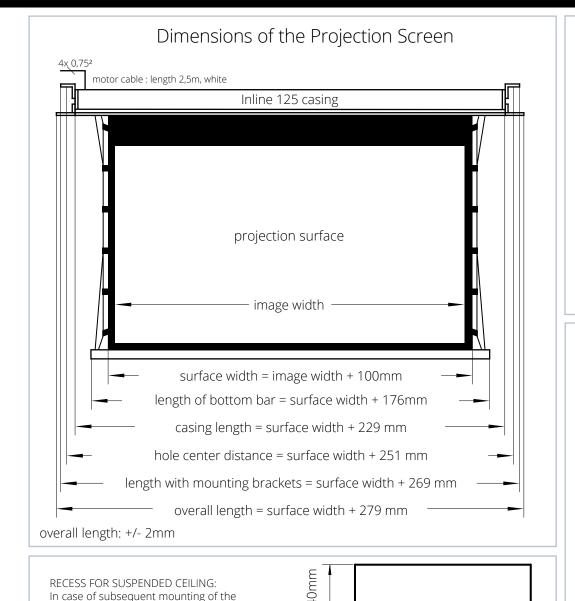
projection screen into a suspended ceiling, a recess according to the sketch has to be made.
