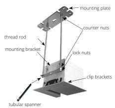
All projection screens in system Inline are available as projection screens for ceiling integration. The clip-brackets on both sides of the screen are detachable to allow convenient access to the screws for mounting and servicing. Mounting and dismounting of the projection screen can be done without service flap.
