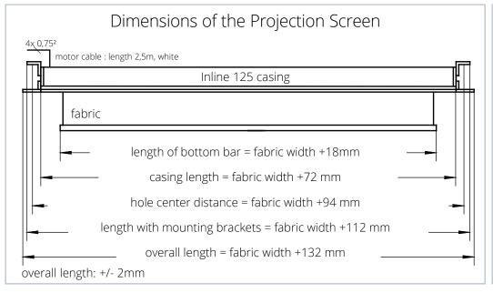
All projection screens in system Inline are available as projection screens for ceiling integration. The clip-brackets on both sides of the screen are detachable to allow convenient access to the screws for mounting and servicing. Mounting and dismounting of the projection screen can be done without service flap.
