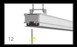
**12:** The projection screen is then attached on each of the two thread bolts in the CEILING CASE with a washer and a lock nut (red). Please make use of the tubular spanner again.
