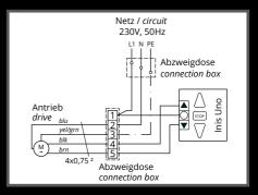
IN ORDER TO AVOID AN ELECTRICAL OVERLOAD OF THE LIMIT SWITCHES IN THE TUBE MOTOR, THE WIRING AND THE CONTROL COMMANDS ,MUST COMPLY WITH THE FOLLOWING REGULATIONS:
