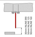
2. THREAD RODS Screw in the thread rods and shorten them according to the sketch.
