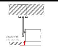
5. CLIP BRACKET Final work will be to close the two lateral gaps with the clip brackets.
