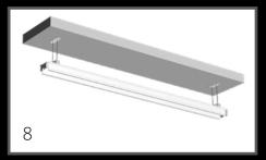
**6-8**: The CEILING CASE is to be adjusted to the intended level of the suspended ceiling by four safety nuts M5. Therefor make use of the delivered tubular spanner.
