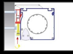
The screen casing (blue) has to be hang up at the rear recess onto the hook profile (red).
