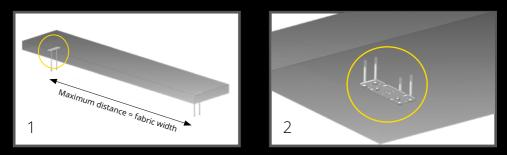
**1-2**: Parallel and aligned mounting of the two ceiling plates with four screws each. (maximum distance = fabric width)
