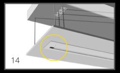
**13-14:** Finalizing, the two lateral gaps are closed with the clip brackets.
