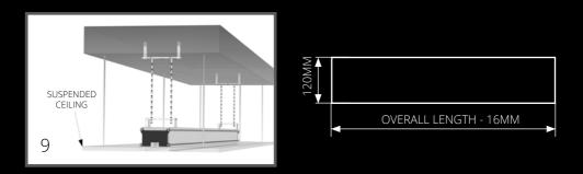
In case of a subsequent mounting a recess according to the sketch above has to be made. overall length = fabric width + 152 mm
