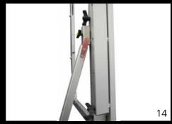
**13-14** Now, connect the projector arms to the three middle struts at the appropriate screwing points with two wing screws M8x85mm each.
