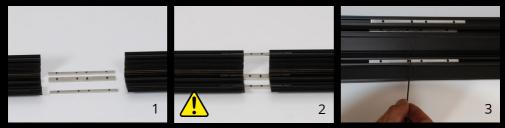
In case of divided profiles, linear connectors are used to join them.Slide in the connectors each half the length in the corresponding slots of the two to be connected frame elements. Put the profiles together without a gap and fix them with the enclosed allen key at the hexagon socket set screws.
