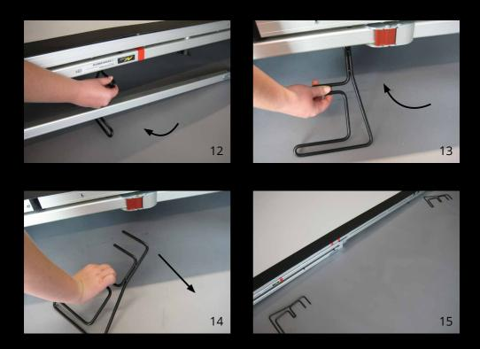
12 - 15 After having attached the legs to the frame the holders have to be removed by rotating them according to the pictures by  $90^\circ$ .
