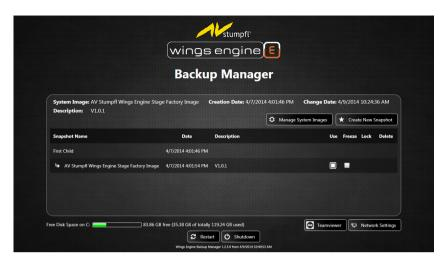
The system initially comes with two snapshots. A **First Child** which cannot be edited and corresponds to the factory setting. Derived from the **First Child** is the **AV Stumpfl Engine Factory Image**, which is the first editable snapshot.
