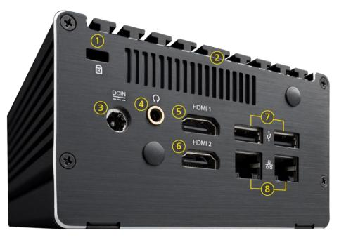
Details to @: The cooling fins act as passive cooling for the dustproof case.
