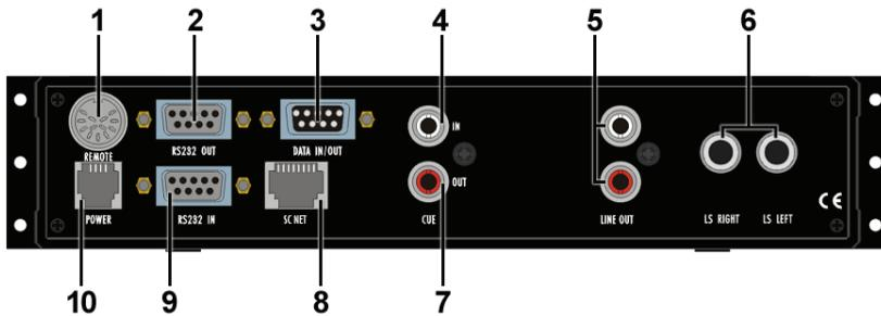
1. REMOTE connector for connection of accessories, such as a cable-operated remote control unit, external IR receiving diode, query switches, Radio Clock Module, cable for DMX or DALI, output of two OC switches (not all of them can be run at the same time!).
