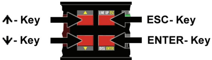
To enter the menu, press both keys ESC and ENTER simultaneously. The display will show "-Menu-". Confirm with the ENTER key and the main menu opens up. The arrows to the right of the menu name indicate the following:
