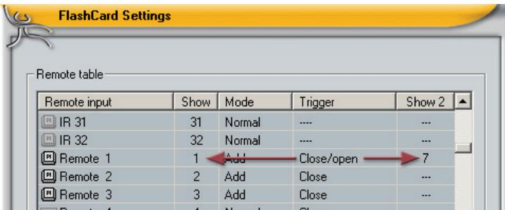
In the example above show 1 is started when the contact closes, while show 7 starts when the contact is opened.
