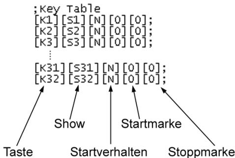
**K1...32** addresses the corresponding key on the IR remote control unit
