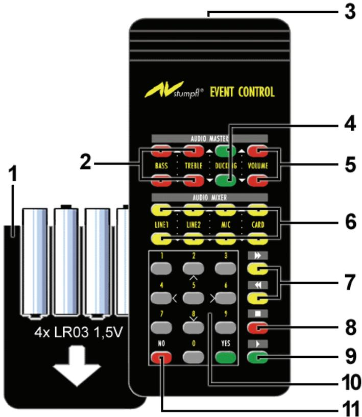
1. Cover of battery compartment, on the rear. **Caution:** Strictly observe the correct polarity indicated at the bottom of the battery compartment when inserting the batteries!
