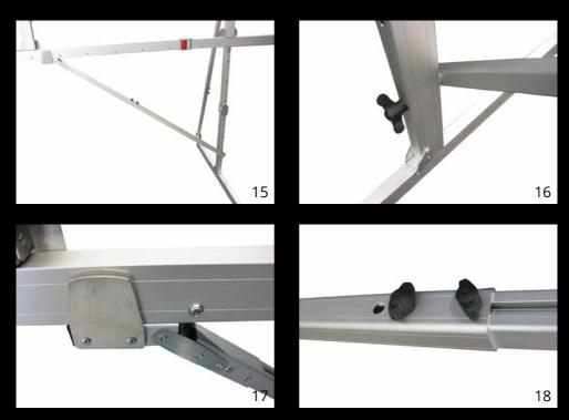
**15-18** Maximum lateral-stability is gained by mounting the anti-sway-braces. Attach the Anti-sway brace through the vertical leg element and open the two wing nuts to be able to adjust the telescopic length and clamp the plates to the horizontal bottom bar of the Monoblox64 screen. Secure the telescopic element and at last thighten the wing screw M8x85mm.
