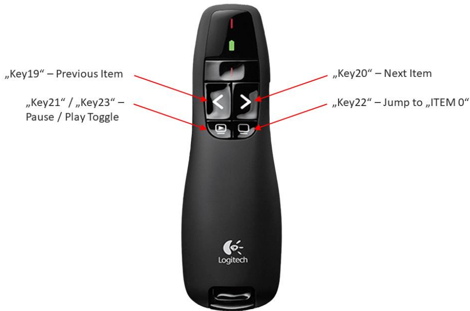
Fig. 56: The Logitech R400 Presenter with default key assignment
