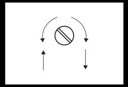
**4** The stop point for the upper emergency limit switch is set by means of the set screw at the second switching cam (green).
