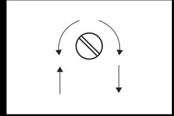
**5** The stop point for the lower emergency limit switch is set by means of the set screw at the lower switching cam (red).
